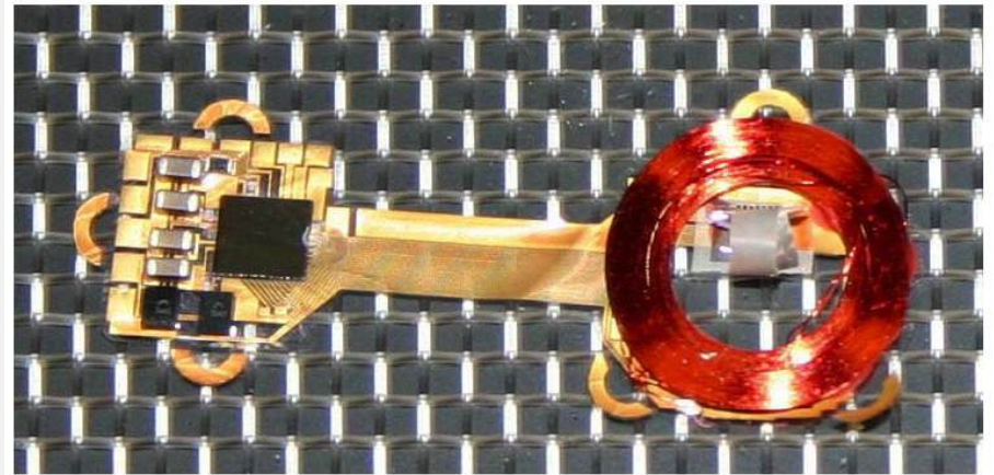
Prototype assembly of an implantable retina : D. Baldwin, et. al, Engent; D. Shire, VA/Boston Retinal Implant Center
